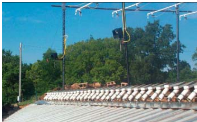
Controlled field testing used this test bed and rainfall simulator to test extreme conditions for silt fence deployed in the field (Fig. 1).
